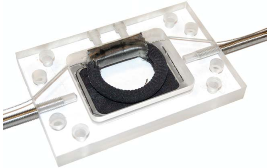
Figure IV-4: Dynamic annulus from the ventricular side. The braided steel wire controls the degree of dilatation of the annulus ring. The wire itself, after setting the right diameter of the annulus, is fixed to the rods that are protruding to the side via a screw mechanism.
